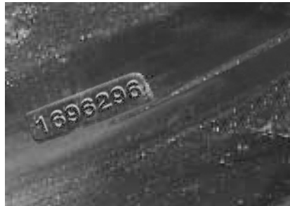
Figure 28. Runflat Serial Number Location
