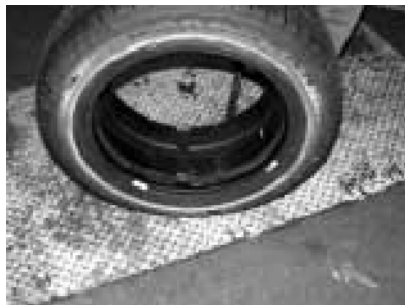
Figure 37. Aligning Runflat with Tire Beads
