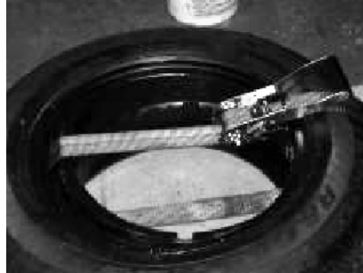
Figure 19. Pressing Ratchet Against Tire Bead
