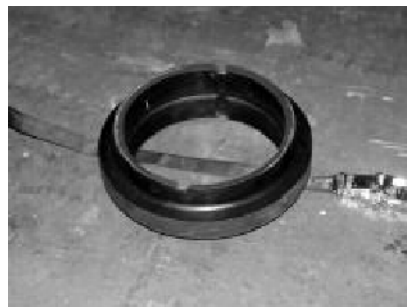
Figure 29. Preparing to Compress Runflat
