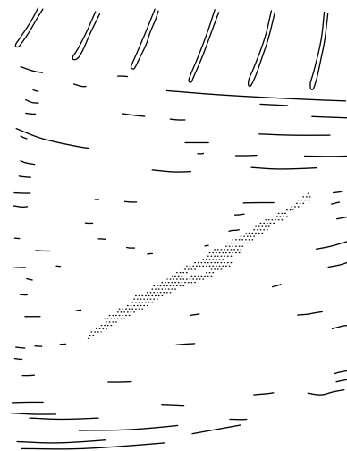
TEAR IN BEAD AREA
