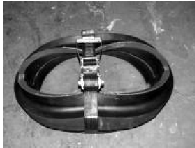
Figure 31. Compressing the Runflat
