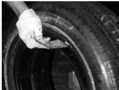
Figure 18. Pulling Strap Over Top of Runflat
