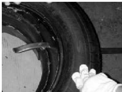
Figure 23. Resting Tire Iron Handle on Hard Surface
