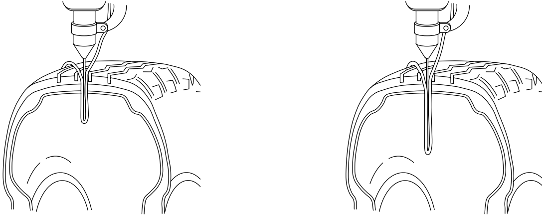
Figure 44. Inserting Repair Material
