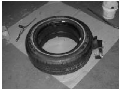
Figure 17. Preparing to Remove Runflat
